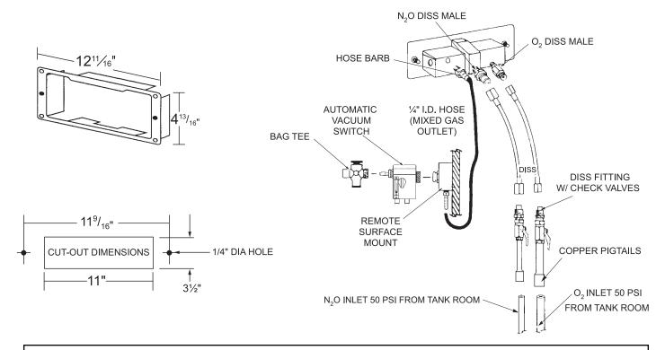
All components are DISS (Diameter Index Safety System) and interchangeable to accommodate the maximum number of installation requirements.
